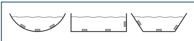
Sensors can be positioned across the channel to capture variations in flow velocity. One of the sensors is also used to measure level so it must be mounted at the bottom of the channel parallel to the water surface.
