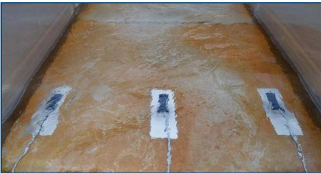
Channels greater than 2 m (6 ft) width or diameter may have significant variations in velocity across the channel width. By mounting three velocity sensors an average velocity profile is measured. The AVMS 5.1 will automatically factor out zero readings at low flow rates if one or more sensors are not submerged or become covered in sediment.
