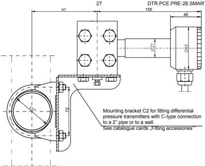
Fig.14. Example: how to install the PRE-28.SMART transmitter on a vertical or horizontal pipe.
