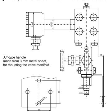
Fig.15. Example: how to install the PRE-28 transmitter with a valve manifold to a wall.
