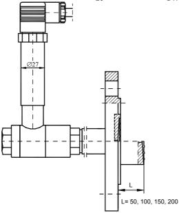
Fig.12. PRE-28.SMART differential pressure transmitter with a single direct diaphragm seal.
