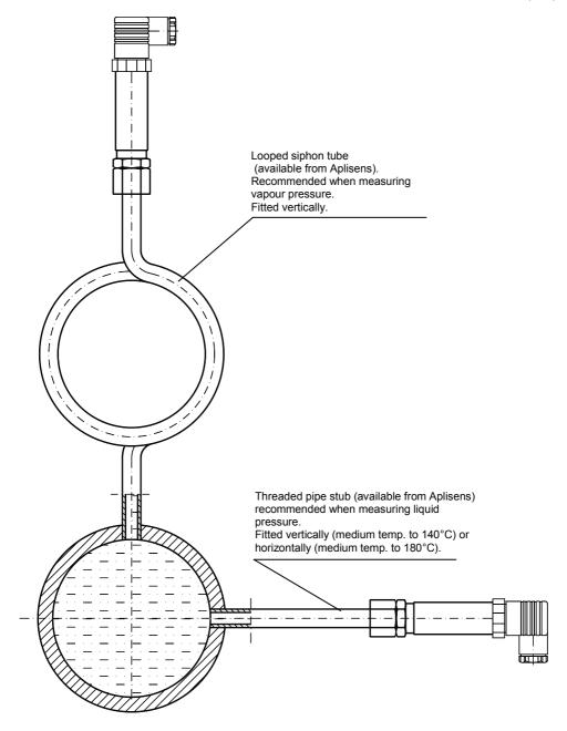
Fig.16. Possible methods of isolating the transmitter from high temperatures.
