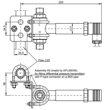
Fig.13. Example: how to install the PRE-28.SMART.
