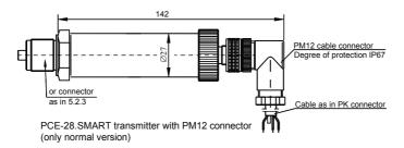
Fig.3. PCE-28.SMART pressure transmitter with PD, PK SG, PM12 connector.
