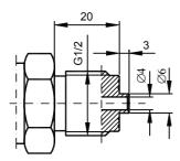
Fig.8a. G1/2-type connector with G1/2" thread
