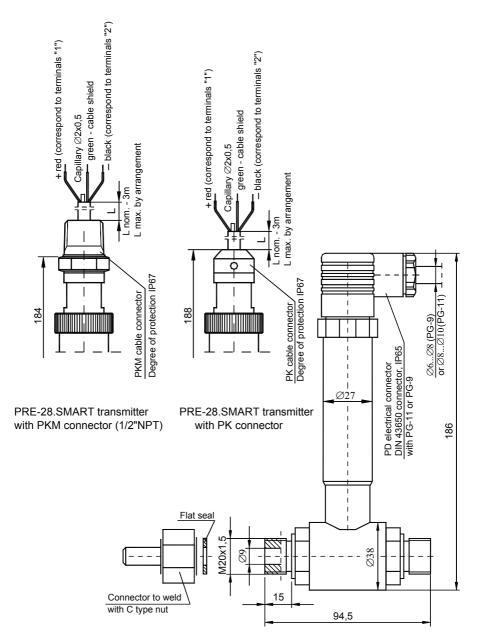
Fig.9. PRE-28.SMART differential pressure transmitter with PD, PK connector.
