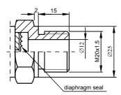
Fig.6a. P-type connector with M20x1.5 thread
