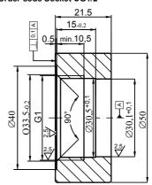
Fig.8f. Weldable fitting ring for use with transmitters with CG1 - type connector Material – 316Lss
