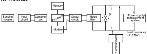
Fig.1. PCE-28.SMART series transmitters - block diagram.
