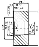
Fig.8d. Weldable fitting ring for use with transmitters with CG1/2 - type connector Material – 316Lss
