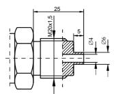
Fig.5a. M-type connector with M20x1.5 thread
