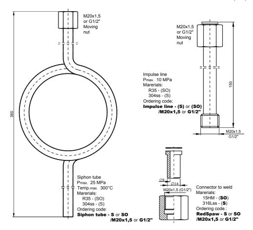
Fig.17. Additional equipment for fitting of pressure transmitters.
