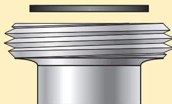
**DIN 11851, size 50mm connection with a gasket**
