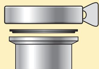
**Tri-Clamp, size 2" connection with clamp and gasket**
